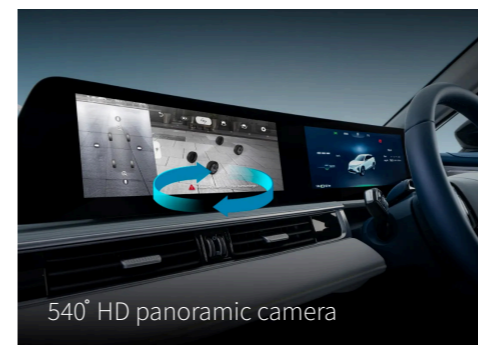
24.6 inch curved screen 3000R with a resolution up to 1920x720
